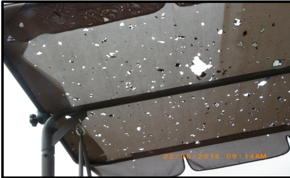
Burn Holes in Canopy of Porch Glider – Ft. McMurray
